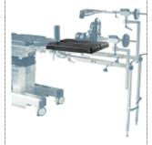
PAIR OF TRACTION LEG SUPPORTS FOR OPT 30/1-**40/1** Legs section for traction support with sphere graft. Not tiltable. Advised for lower limbs traction device code 9923046.
